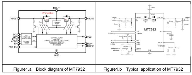
MT7932 features high voltage and current rating at 33V and 5A, integrated 25mOhm ultra-low Rdson power devices with loss-less current sensing and analog current reporting. MT7932 provides comprehensive protection functions including Input voltage surge protection; Input current surge protection; Output constant-current control; Output short-circuit protection; Thermal shutdown
