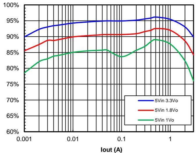
**5V Input 3A 1.5MHz Synchronous Step-Down DC/DC Converter**
